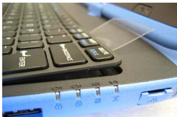
Insert the first card on height of the „Insert“-Button between casing and keyboard.
